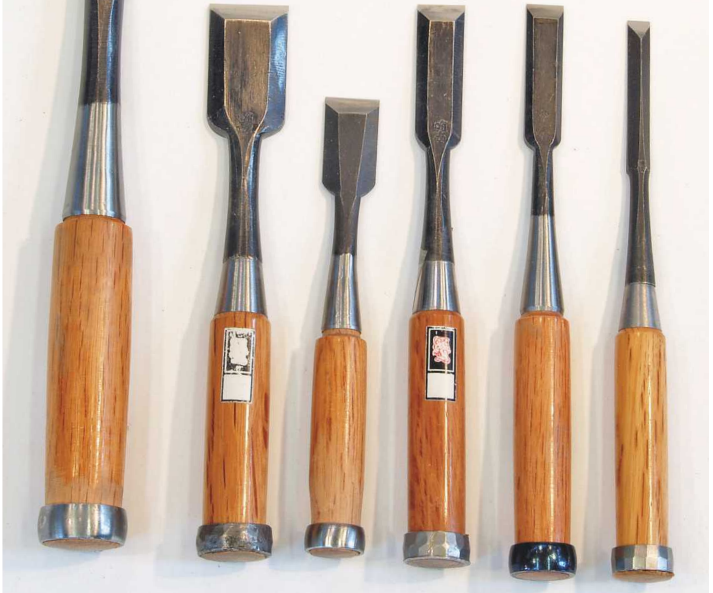
Pic.5 Oire nomi: these are standard bench chisels
